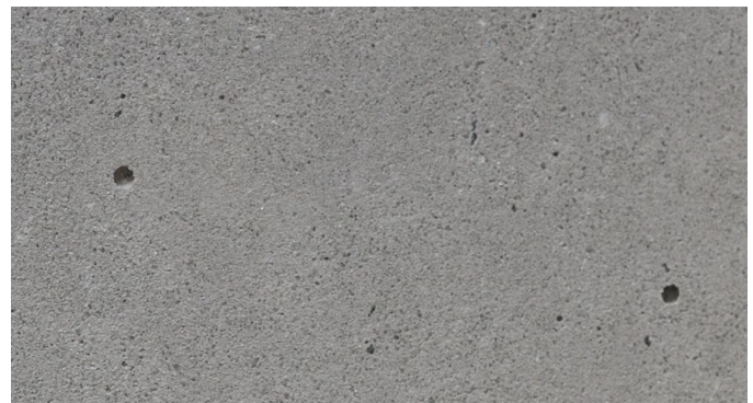
1/8" diameter pores in an Acid Wash finish
