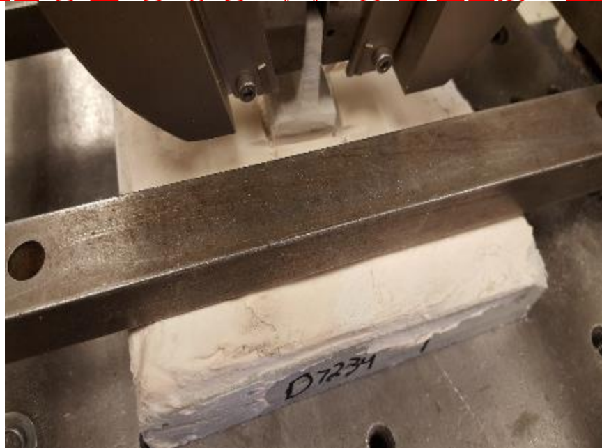
Photo No. 2 ASTM D7234 Pull-off Strength - Latapoxy 310 with GFRP Failure Mode
