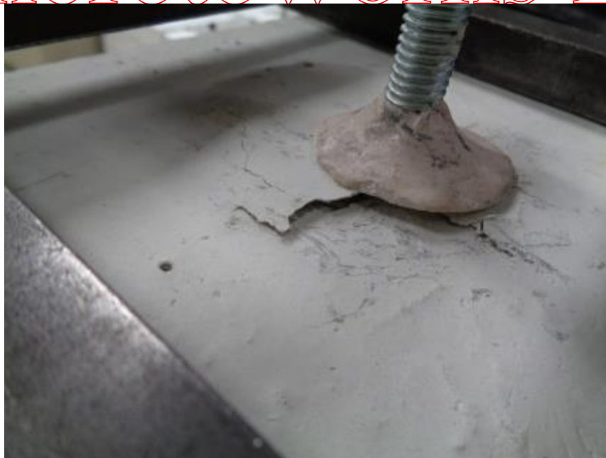
Photo No. 6 ASTM E488 Tensile Anchor Load - Embedded Threaded Rod Failure Mode
