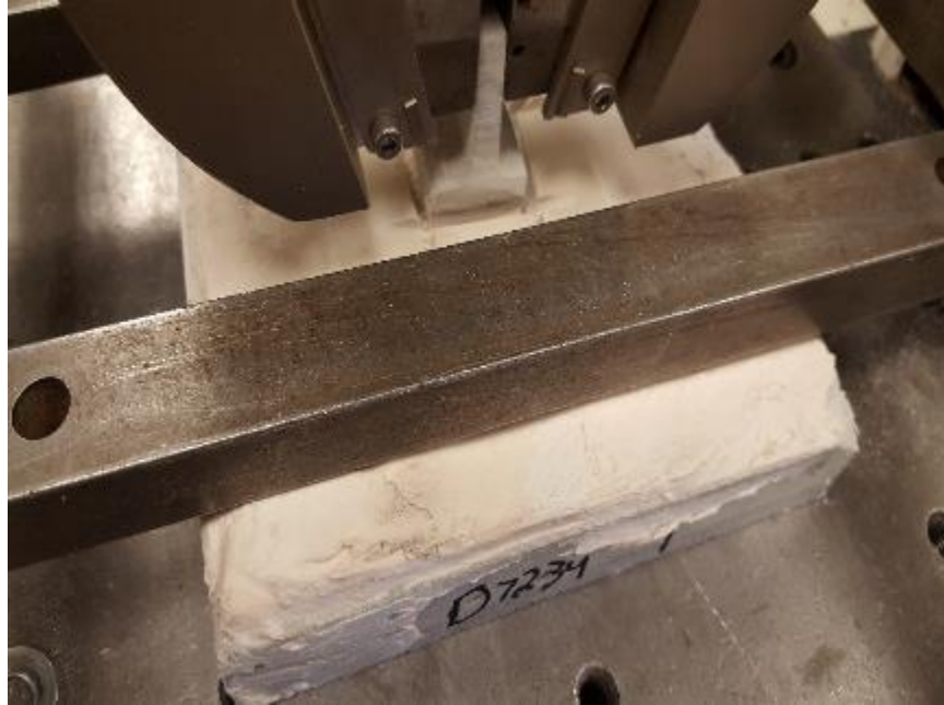
Photo No. 1 ASTM D7234 Pull-off Strength - Latapoxy 310 with GFRP Test Set-Up
