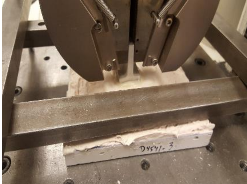
Photo No. 3 ASTM D4541 Pull-off Strength - Latapoxy 310 with DensShield Test Set-Up
