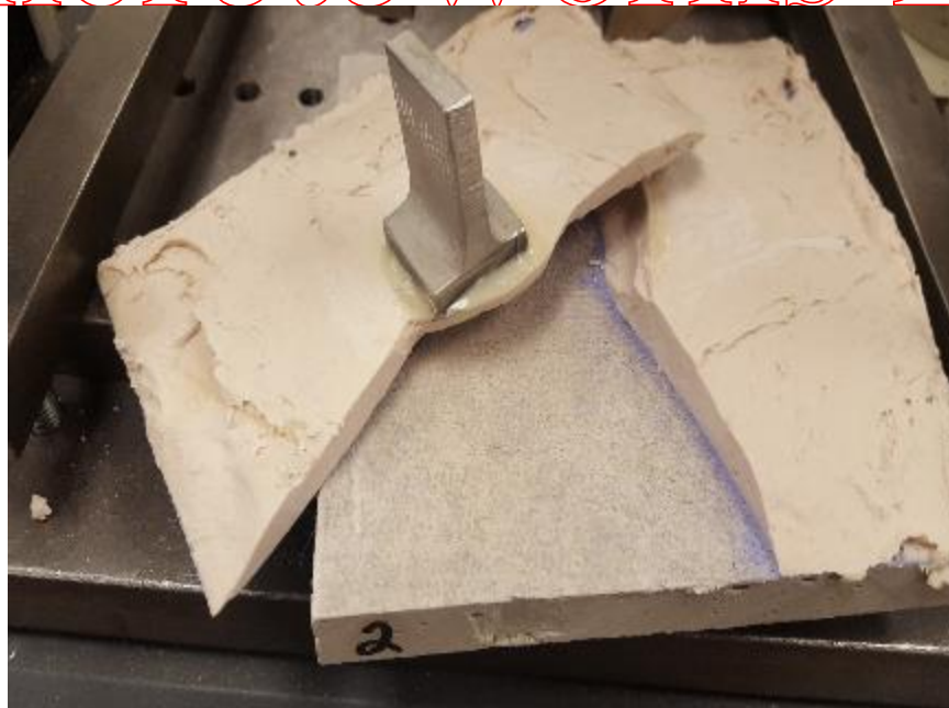
Photo No. 4 ASTM D4541 Pull-off Strength - Latapoxy 310 with DensShield Test Set-Up
