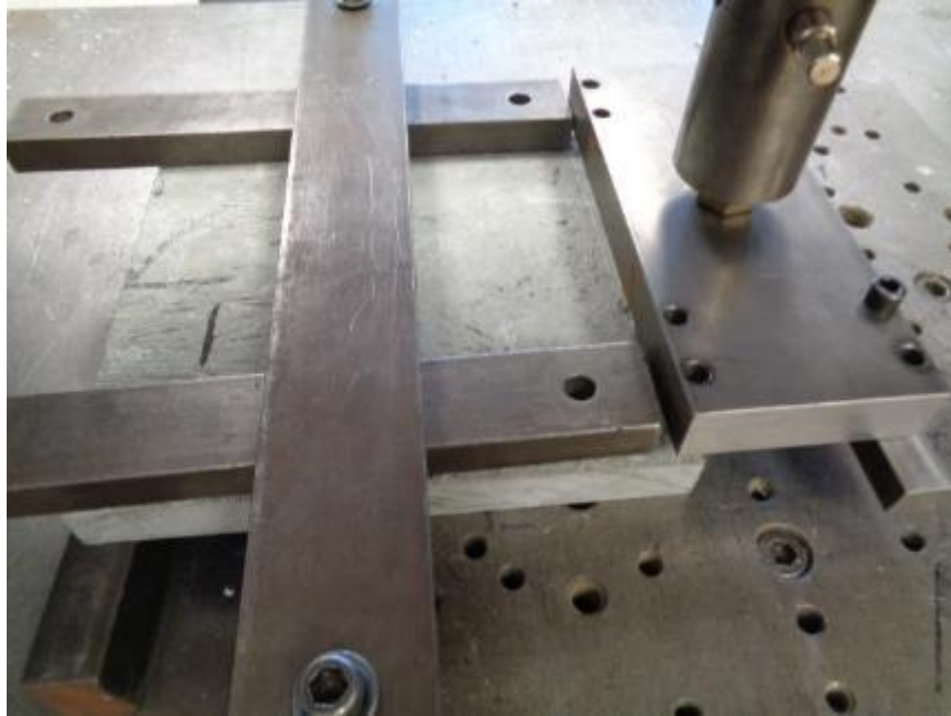
Photo No. 7 ASTM E488 Shear - Embedded Mechanical Clips Test Set-Up
